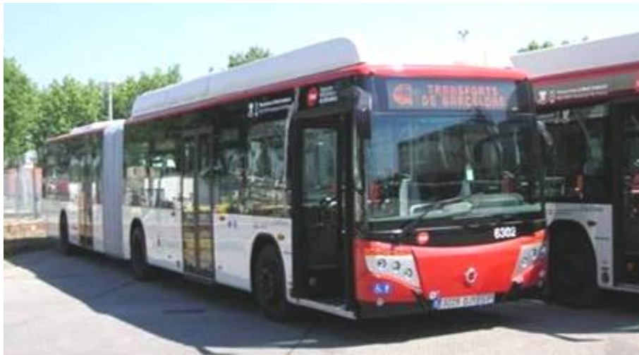
Irisbus Iveco CITYCLASS CNG 12 & 18 m 280 CV. Stoichiometric turbo engine. EEV certified
